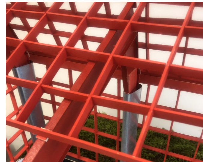
Fig.18 1:20 scale model of "The Urban Farming Project." This model shows in detail the metal structures used for vegetable production. In this structure, the plants rotate across three levels. At the bottom, the plants absorb water from large tanks, while at the top, the plants are exposed to sunlight.
