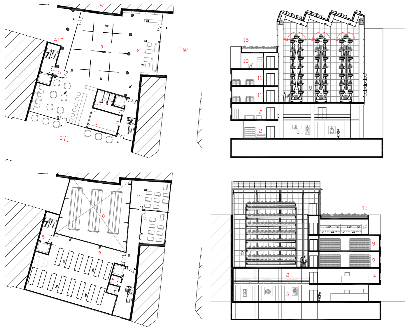
Fig.14 Ground floor and second-floor plans of “The Urban Farming Project.” The ground floor is focused on cultivation, with a restaurant and an art gallery. The second floor is dedicated to soilless agriculture. To allow the two programs to operate in synergy, the thresholds have been separated: the threshold for production is in the building’s backyard, while the threshold for cultural activities faces one of the main streets.
